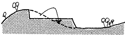
CUT = FILL FOR BUILDING PLATFORM
