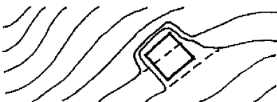
NOTCH FOR BUILDING PLATFORM
